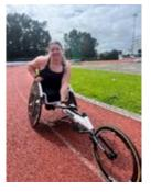
in a straight line, and are aerodynamically designed to enhance track performance. Racing wheelchairs should be custom made to fit the user's body. Throwing frames are individually designed assistive devices which are scaffold¬like chairs made of metal bars and plates welded together customised to the athletes. Throwing frames are secured to the ground inside a throwing circle by straps allowing no
